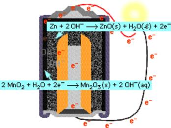
Nearly same reactions as in common dry cell, but under basic conditions.
