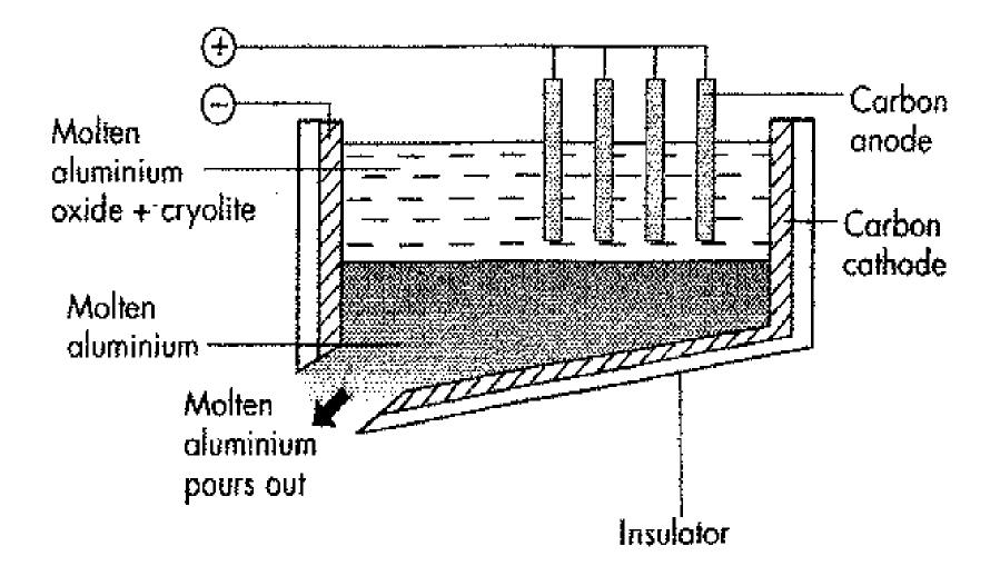
Figure 1: Extraction of aluminium by electrolysis of bauxite
